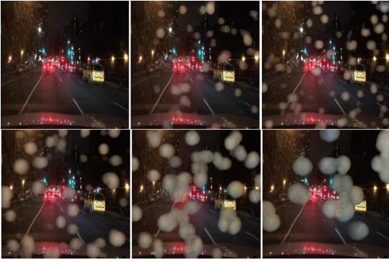
Fig. 3. Generation of synthetic rain images conditioned on input.
