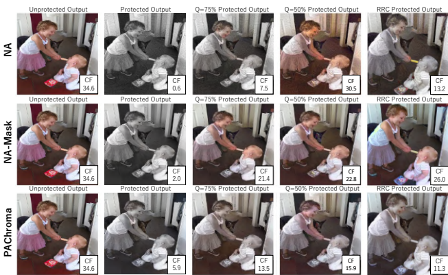
Fig. 5. Robustness of NA, NA-Mask, and PACHroma to JPEG compression ( Q=X\% ) and Random Resized Cropping (RRC). Each image is shown with its CF score on the bottom corner.
