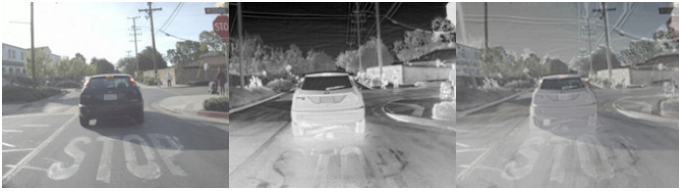
Fig. 1. Misaligned infrared and visible images from the RoadScene dataset. From left to right are a visible image, an infrared image, and a fused image by SuperFusion.
