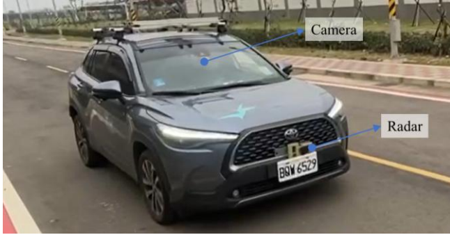
Fig. 9. The testbed with equipped sensors.
