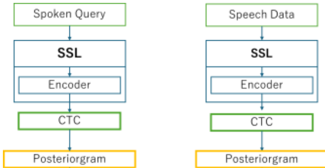
Fig. 2 proposed method: posteriorgram matching using a model with a CTC layer attached to the output of SSL encoder
