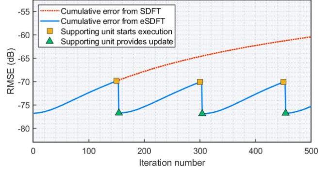
Fig. 2. RMSE comparison under single-precision floating-point format with window length N = 1024 . eSDFT successfully bounds the error near -75 dB by invoking supporting unit updates. Classical SDFT accumulates error over iterations due to finite-precision limitations.
