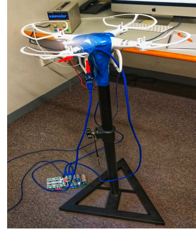
Fig. 3. Experimental Setup, with microphone array attached to the body of drone closer to the selected motor.
